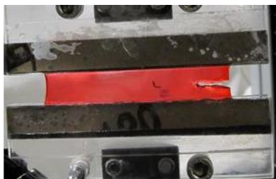
Typical “pure shear” experiment for fracture of hydrogels developed in the laboratory.
