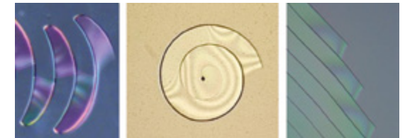
Different morphologies of thin film cracking.
