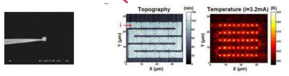
Left : SEM image of a fluorescent-SThM tip; Right : topography and thermal images measured on a nanostructured microwire, hot spots are visible at every constriction.
