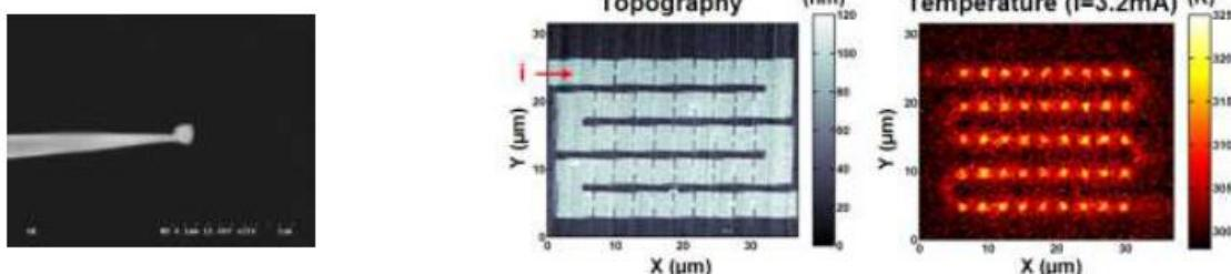
*Left : SEM image of a fluorescent-SThM tip; Right : topography and thermal images measured on a nanostructured micro-wire, hot spots are visible at every constriction.*
